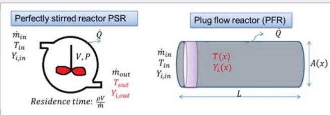
F1: PSR describes highly turbulent-mixed reacting flows (L). PFR: Describes unidimensional reacting flows (R)
