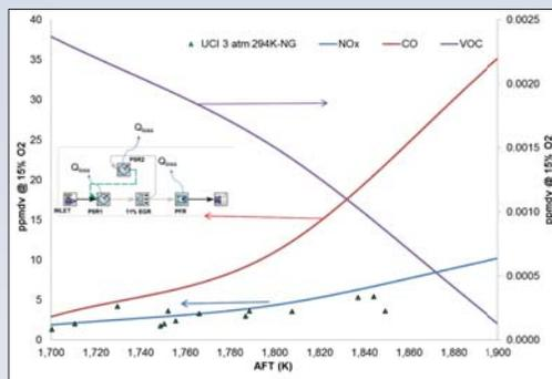
F3: Prediction of NO<sub>x</sub>, CO and VOC using CRN. Comparison with experimental NO<sub>x</sub> data at 3 atm.
