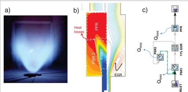
F2: a) Characteristic low swirl reaction. b) Classification of the zones using CFD results. c) Equivalent CRN
