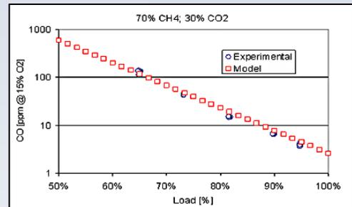
Figure 3: Model and experimental data comparison
