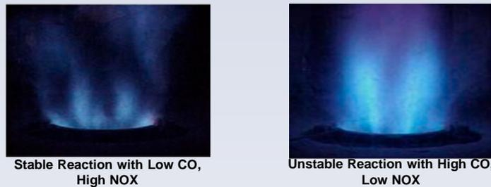
Figure. 1 Burner Running Conditions
