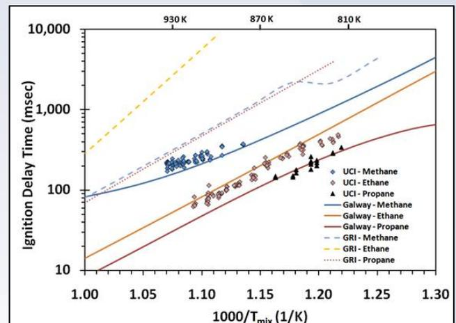
Figure 3: Comparison of chemical mechanisms to experimental ignition delay results
