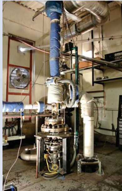
F2: Clockwise from Left: Test Apparatus, Reverse Step Flameholder, Cylindrical Flameholder, Natural Gas Flame with Cylinder, Natural Gas Flame with Reverse Step
