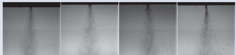
F3: High Speed Images (L > R): F-76, BE60, Ethanol, Methanol
